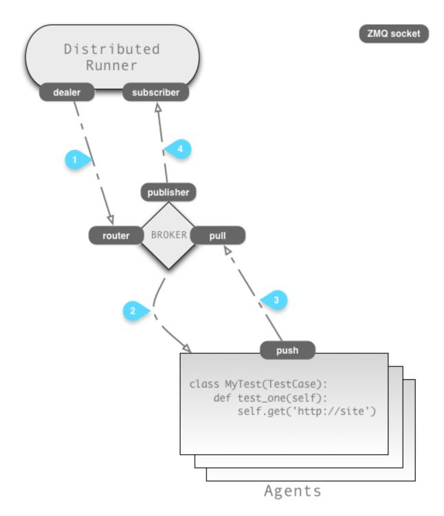
All the communication is handled through ZeroMQ sockets, as you can see in the diagram.
